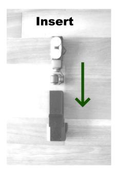
When removing, grab by the exposed body as shown, push inwards and pull straight up as vertical as possible.
